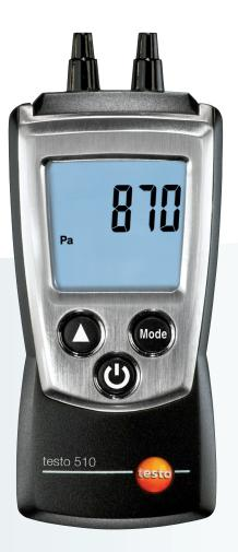
The testo 510 is very handy, small and easy to operate. It measures differential pressure in a range of 0 to 40 inH2O. The differential pressure measurement is temperaturecompensated for accurate measurement values which can be displayed in Inches of Water Column over the entire measurement range. Magnets on the back of the 510 permit free-hand work. The backlit display allows the measurement values to be easily read out, even in unfavorable light conditions.
